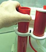
There is a small screw at the edge of the wedge shaped tube holder with which the wedge shaped tube can be clamped into the guide holder.
