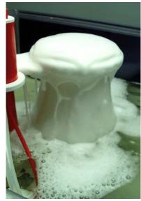
Let the skimmer run for several hours without placing the pot on top.
