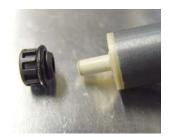
If the rear bearing brush – as seen on the photo – sits on the shaft when removing the impeller unit, it is vital to carefully remove the bearing from the shaft photo
