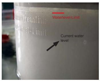
On the figure you can see the water level stripline approx. 5 cm below the maximum level. This water level stripline can be lowered or rised by turning the tube.
