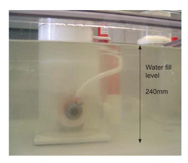
Depending on how high is the water fill level in the filter, the Bubble King® Double Cone can be placed on the right height, to achieve an optimal result of skimming.
