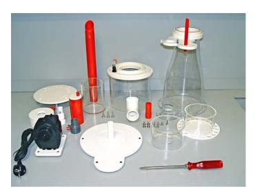
Remove all parts which can be dismantled, such as the wedge shaped tube, pot, hose, pump and also the T-piece from the outlet, including all titanium screws. Pull out the red pipe for injection using a sharp tong.
