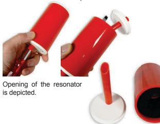
Now, the silencer inlay can be washed out with fresh water. The inlay must be **completely dry** before reinstalled again!
