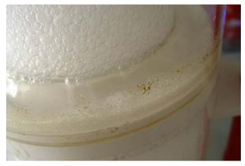
Please keep the skimmer running until the absorbate pot (skimmer head) has been filled by a foamy liquid.
